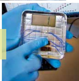
A generator that uses viruses to turn mechanical energy into electricity, right, was developed by Berkeley researchers Byung Yang Lee , Seung-Wuk Lee and Ramamoorthy Ramesh , above.
